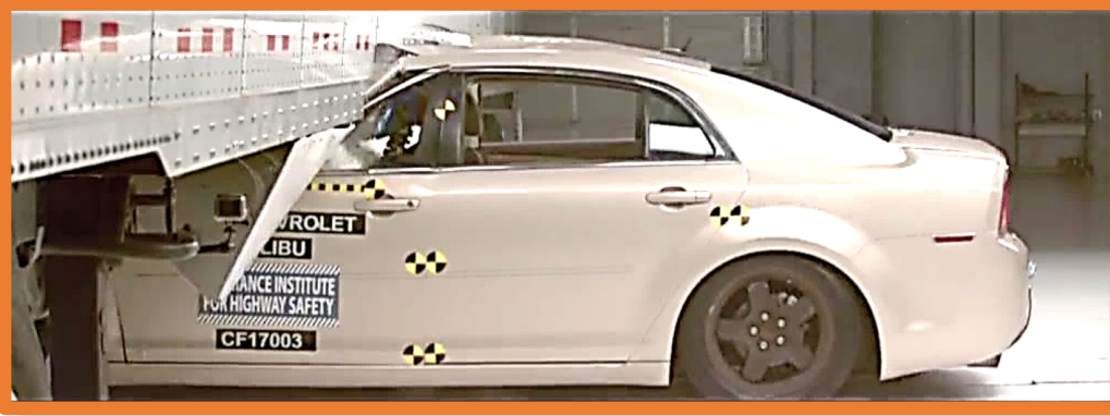
Fatal Crash WITHOUT AngelWing (aero-skirt only) 35mph
